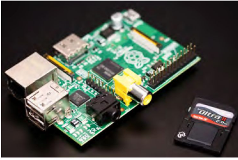
Fig. 2. A Raspberry Pi, without any attached connections. I/O headers are at the bottom right, and the Ethernet connection is on the top left. The system runs off an SD memory card, which contains the operating system.
