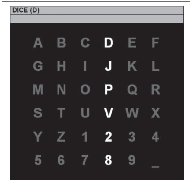
Figure 1. The 6 \times 6 matrix used in the current study: a row or column flashes for 100 ms every 175 ms. The letter in parentheses at the top of the window is the current target character “D.” A P300 should be elicited when the fourth column or first row is flashed. After 15 flash sequences (ie, each row and each column has been flashed 15 times), the collected brain responses are processed and classified, and online feedback is provided directly below the character to be copied. The process is then repeated for the next target character “I” and so forth until all characters in the word “DICE” have been presented as targets.
