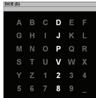
Fig. 2: The 6x6 matrix used in the current study. A row or column intensifies for 100 ms every 175 ms. The letter in parentheses at the top of the window is the current target letter “D.” A P300 should be elicited when the fourth column or first row is intensified. After the intensification sequence for a character epoch, the result is classified and online feedback is provided directly below the character to be copied.
