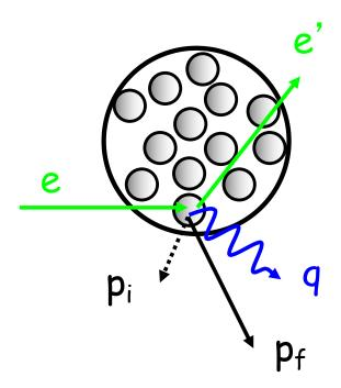
Initial nucleon energy:  $KE_i = p_i^2 / 2m_p$ Final nucleon energy:  $KE_f = p_f^2 / 2m_p = (\vec{q} + \vec{p}_i)^2 / 2m_p$ Energy transfer:  $v = KE_f - KE_i = \frac{\vec{q}^2}{2m_p} + \frac{\vec{q} \cdot \vec{p}_i}{m_p}$ Expect: •Peak centroid at  $v = q^2/2m_p + \varepsilon$
