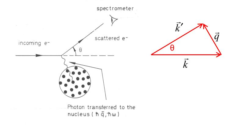
Simple analogy for elastic electron scattering.... Classical Fraunhofer Diffraction
