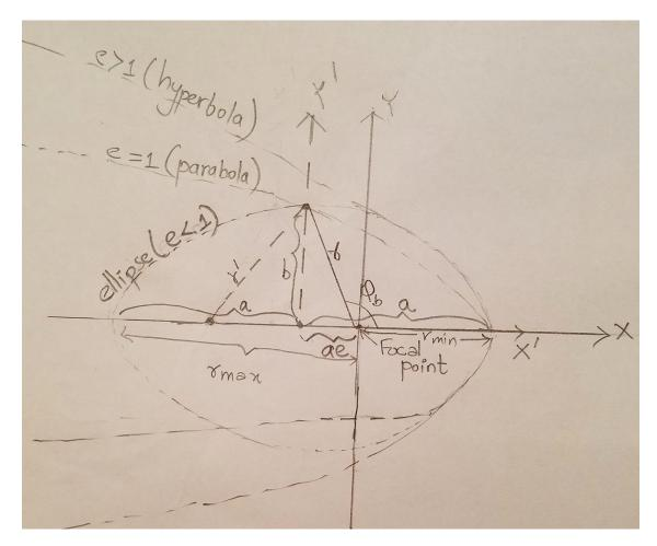
Figure 3: Trajectory of the body with varying eccentricity in the central force field
