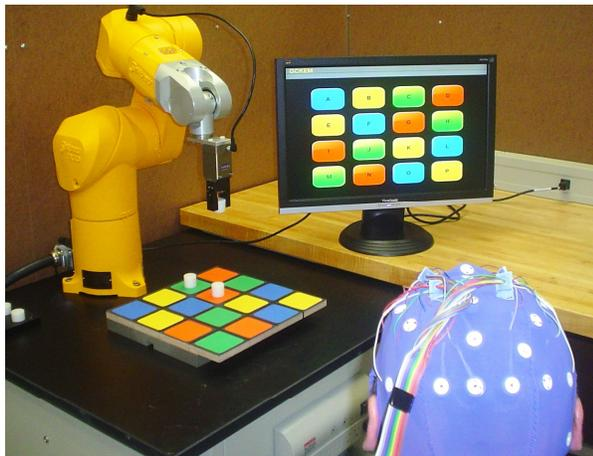
Fig. 3. The Staubli robotic arm and display setup. Note the board colors spatially correspond to the display, allowing the subject to quickly ascertain if the robot placed the block where they intended.
