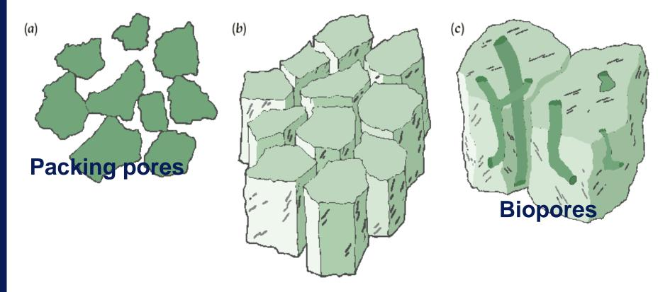
(a) Many soil pores occur as packing pores, spaces left between primary soil particles.
