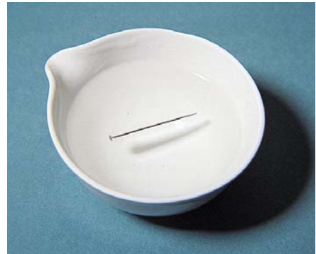
Figure 11.18: A steel pin floating on the surface of water. Photo courtesy of American Color.
