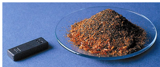
Figure 1.15: A mixture of potassium dichromate and iron filings. Photo courtesy of James Scherer.
