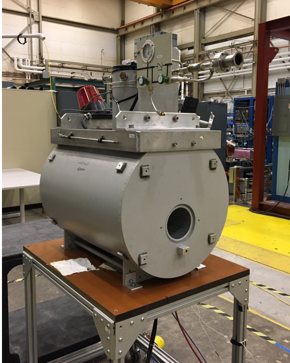
5.0 T solenoid for Hall B Frozen Spin Target (Cryomagnetics, Inc.)
