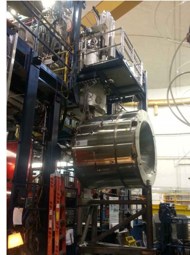
5.0 T Solenoid for CLAS12 (Everson Tesla, Inc.)
