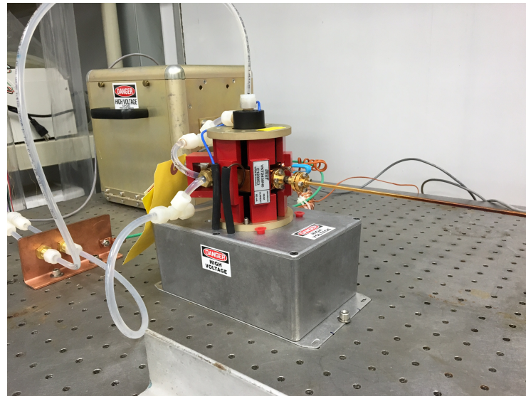
Extended Interaction Oscillator, 20 W @ 140 GHz CPI Canada
