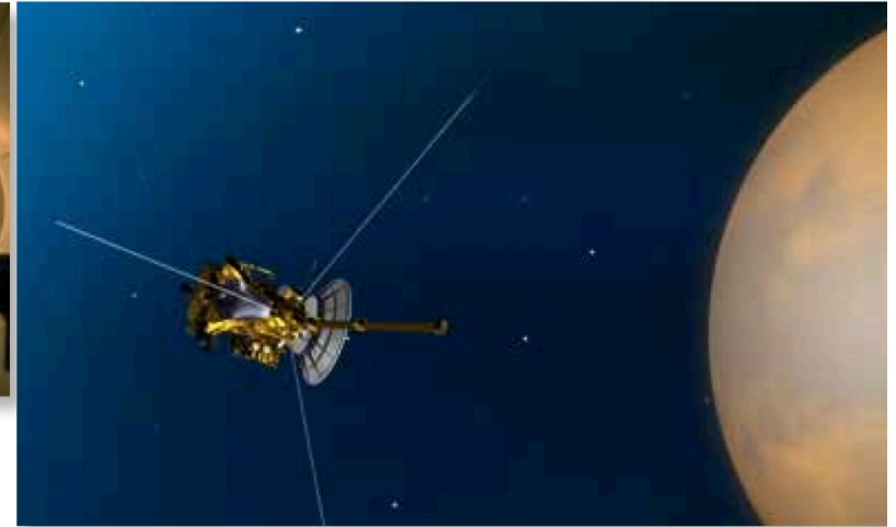
The Cassini spacecraft gets power from plutonium, a nuclear isotope.
