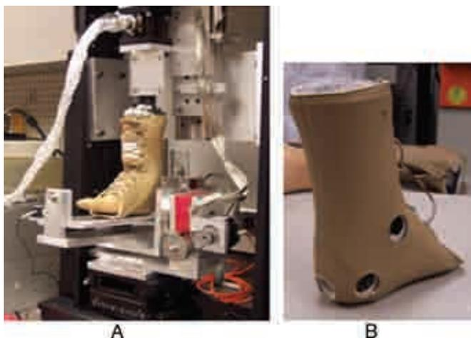
Figure 1. A, Experimental setup for Arizona AFO stiffness testing. B, Arizona AFO modified for gait analysis.
