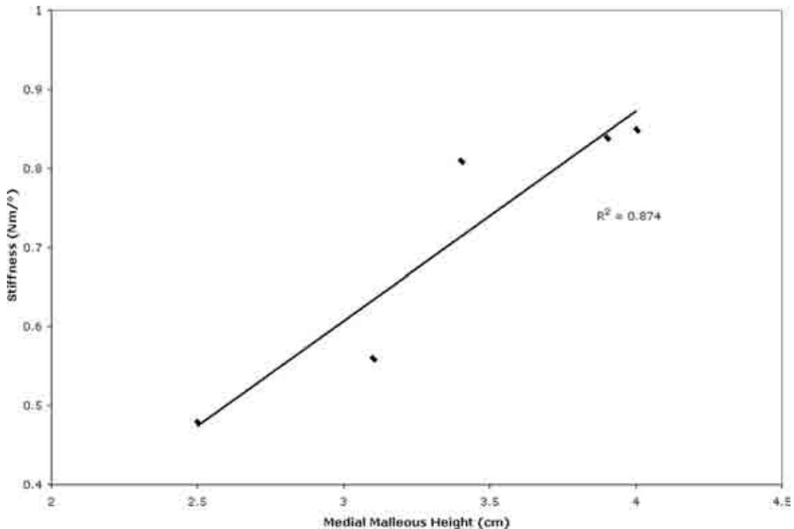
Figure 3. The change in plantarflexion stiffness increased as the height of the medial malleolus increased.
