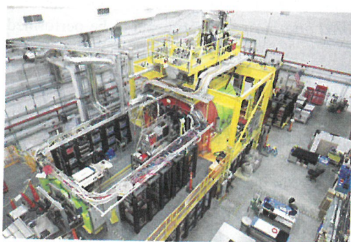
Figure 4. Left: The photo of Hall D shows the solenoid and a platform upstream containing the cryogenic target equipment and electronics racks. Right: the schematic picture of the spectrometer.
