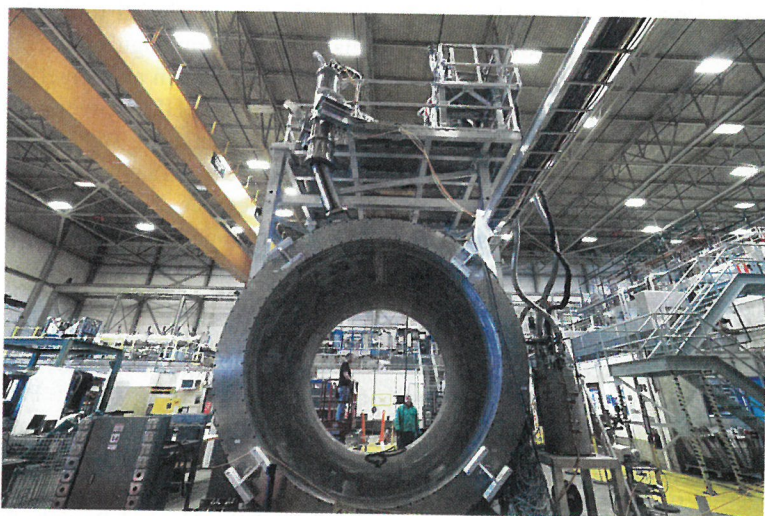
Figure 7. The CLEO-II superconducting solenoid magnet is being refurbished inside the SRF Test Lab for the SoLID detector system to be eventually deployed in Hall A at CEBAF.
