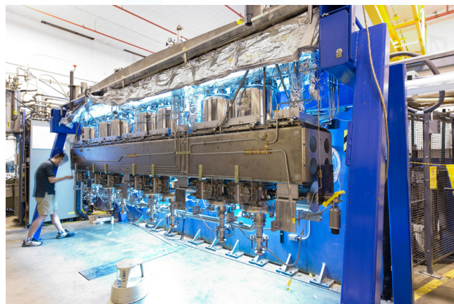
Figure 9.2. ATLAS upgrades. (left): A string of superconducting cavities and focusing solenoids developed for the recent intensity and energy upgrade at ATLAS. (right): The EBIS developed to increase the purity of neutron-rich ion-beams extracted from CARIBU for reacceleration in ATLAS [39].
