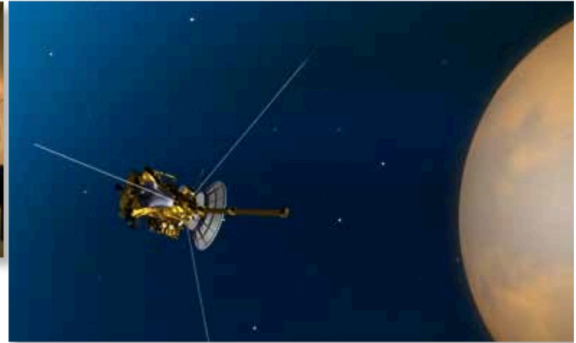
The Cassini spacecraft gets power from plutonium, a nuclear isotope.
