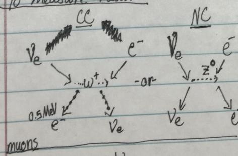
Take an electron (from some atom) and merge it with a neutrino from the sun. Using a gauge boson, the two particles swap types. Doing this causes the new electron to give off Cherenkov radiation (as the new electron is free). The light given off by this radiation can be measured by photodetectors (water is typically used for the source of electrons).
